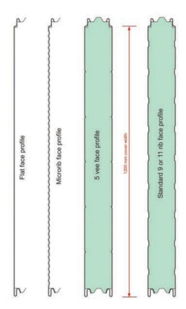
The Isowall panel is supplied with a range of face profile options as shown above. Typically the Microrib finish is specified on panels utilised in external cladding.
